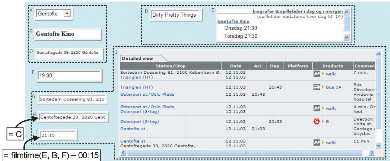
Figure 4: Using three Web applications in combination to provide travel information for film outings. The cell relationships established by clipping from the pages shown as thumbnails at the top are as follows: selecting a cinema in the list in cell A triggers navigation that places the cinema's name and address in B and C respectively; entering a film name in D causes E to hold a list of that film's Copenhagen-area screenings for today and tomorrow; cells G, H and I serve as start address, destination and arrival time for a travel enquiry that gives an itinerary in J. Cell F is an independently created cell in which the user specifies the earliest desired film start time. The applications have been connected by giving cell H (destination) a formula that copies the cinema address from C, and cell I (arrival time) a formula based on a user-written function for finding in cell E the first screening time relevant to cinema name B and time F. Any change to the cinema choice in A, film name in D, earliest start time in F, or starting address in G will trigger re-evaluation leading to a new itinerary.
